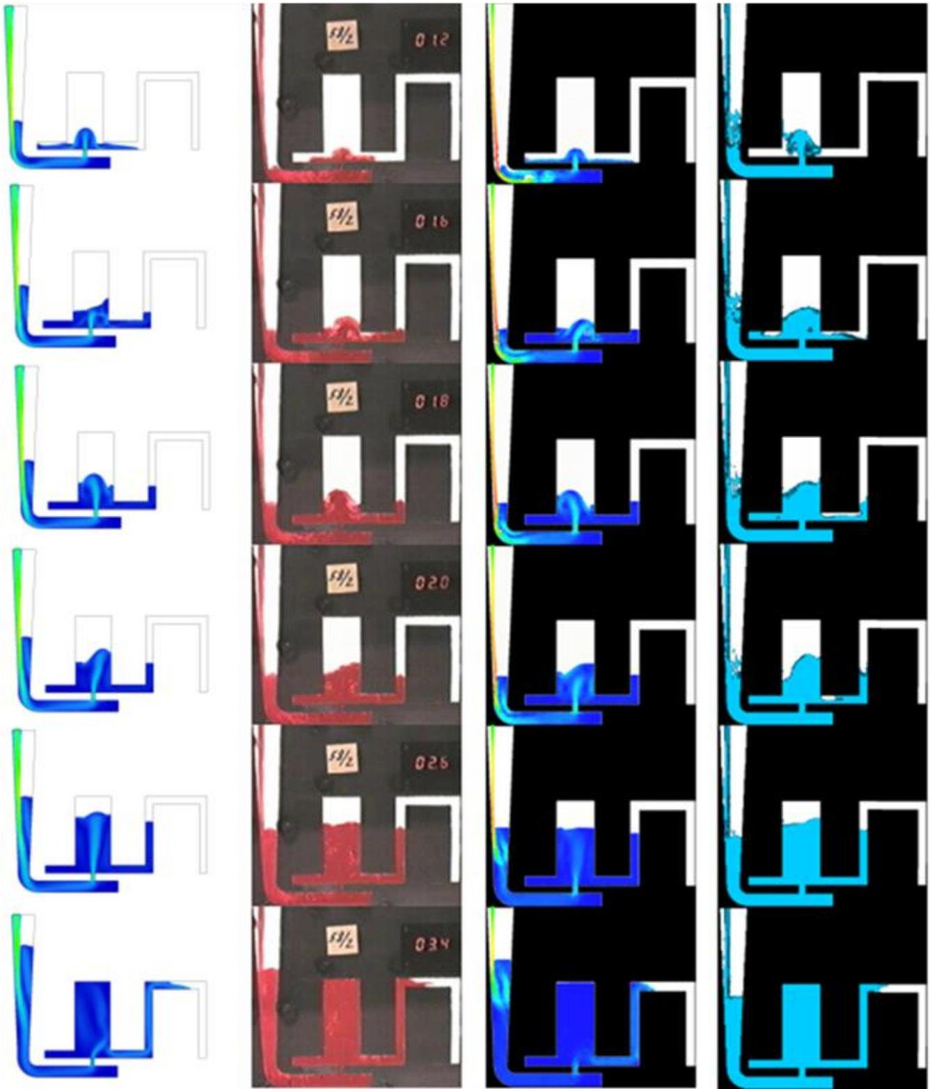
Figure 37. Filling (from left to right): AMS Solver, Experimental (Ha et al. 1999), SPH (Ha et al. 1999) and MagmaSoft (Ha et al. 1999).
