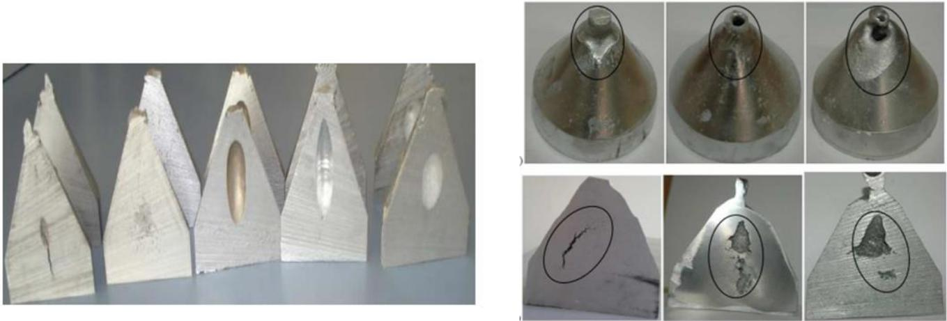
Figure 32. Experimental inner and pipe shrinkage for the Tatur test (left image (Brúna and Sládek 2011); right image (Haj, Bouayad, and Alami 2018)).
