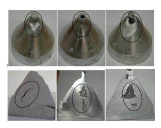
Figure 32. Experimental inner and pipe shrinkage for the Tatur test (left image (Brůna and Sládek 2011); right image (Haj, Bouayad, and Alami 2018).
