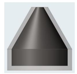
Figure 27. Geometry of the Inspire Cast simulation for the Tatur Test.
